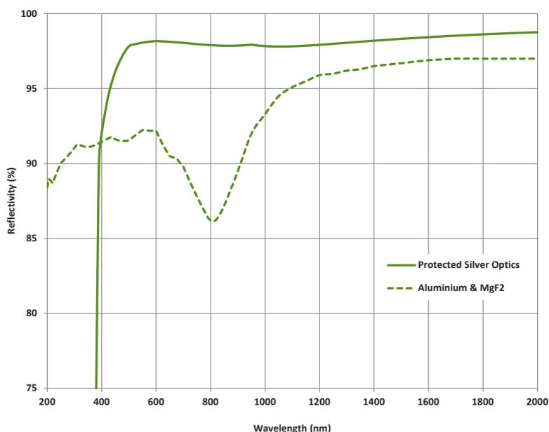
The graph shows the standard Al + MgF<sub>2</sub> optics coatings reflection efficiency versus wavelength.
