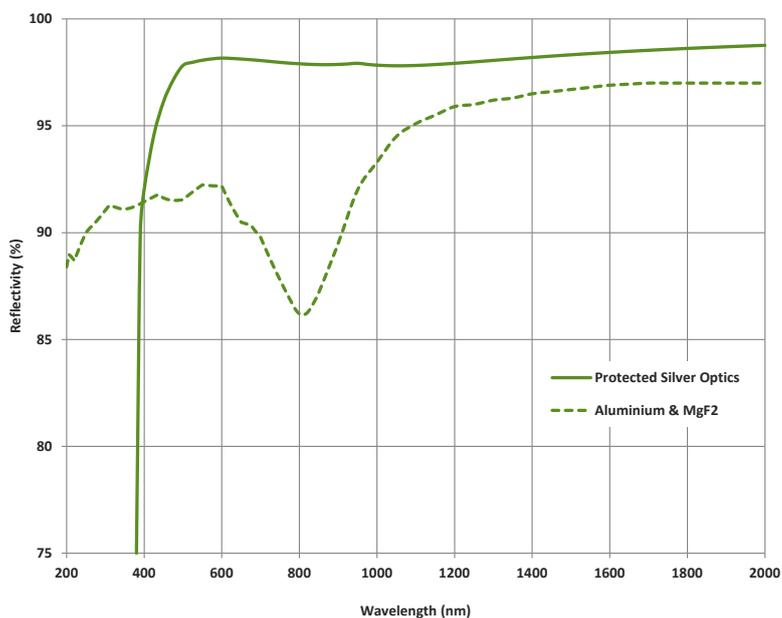
The graph shows the standard Al + MgF<sub>2</sub> optics coatings reflection efficiency versus wavelengths.
