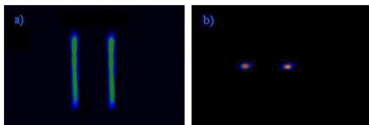
**Figure 1.** Images produced at the exit of the Shamrock 750 with light from a Mercury source (577 and 579 nm lines) and 100  $\mu\text{m}$  core fibre-optic.
