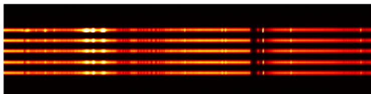
**Figure 2.** Image produced at the exit of the Shamrock 750 with a combination of broadband and Mercury light sources. A 5-way, 100  $\mu\text{m}$  core fibre-optic assembly was used at the entrance of the spectrograph.
